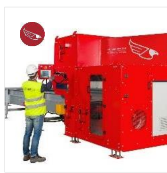
FALCON: NIR (NEAR INFRA RED) OPTICAL SORTER TO ELIMINATE CHLORINATED PLASTICS
