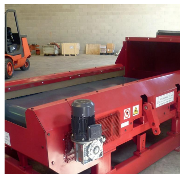
INDUCED CURRENT SEPARATOR, TO RECOVER ALUMINUM, ETC ...
