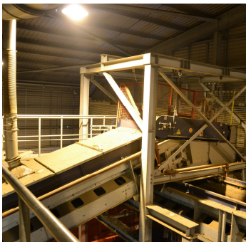
MAGNETIC SEPARATOR TO SEPARATE FERROUS METALS
