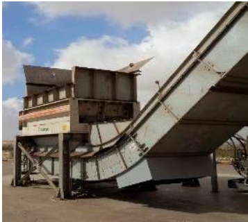
PRIMARY SHREDDER, TO HOMOGENIZE SIZE AND ALLOW BETTER REFINING
