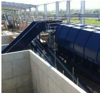
ROTATING DRUM SCREENER TO SEPARATE GRITS AND FINES TO BE LANDFILLED OR USED AS LANDFILL COVER
